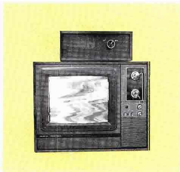
During the subscription television broadcasts, Ch. 52 viewers get a "scrambled" video signal, while subscribers receive a clear picture on channel 6.
