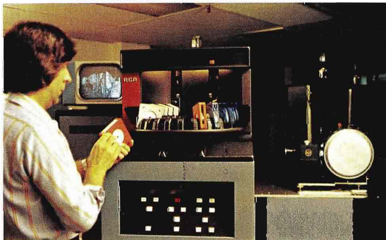
Addition of the cartridge film system freed up one of TV-30's two telecine systems for full-time production use.
