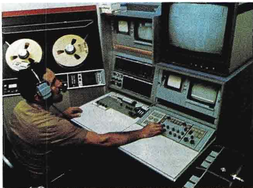
Master Record facility next to the studio area is equipped with a TR-600 tape machine; camera control units, and a basic video switcher.
