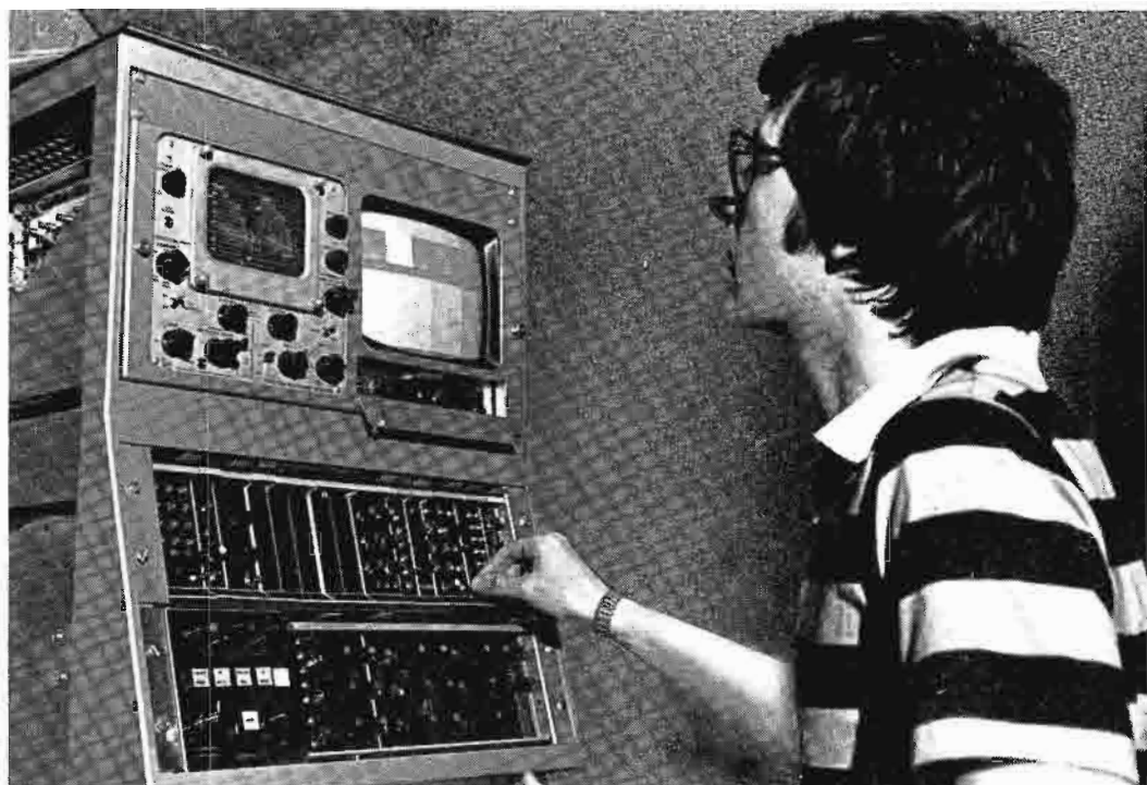
Video module includes control units for three TKP-45's and three TK-44 cameras.
