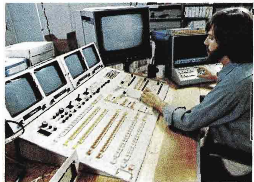
Editing and dubbing area includes three TR-600's, video switcher and computer editing system. Facility operates around the clock during the week to handle dubbing requirements.
