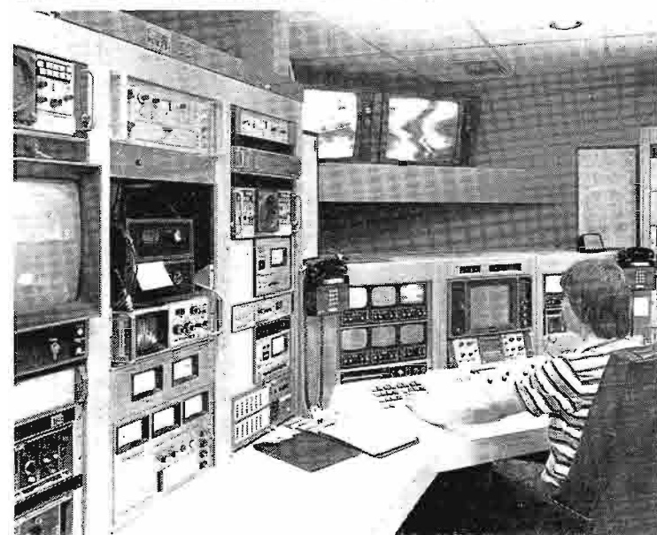
Master Control includes monitor displays of scrambled and unscrambled pictures.
